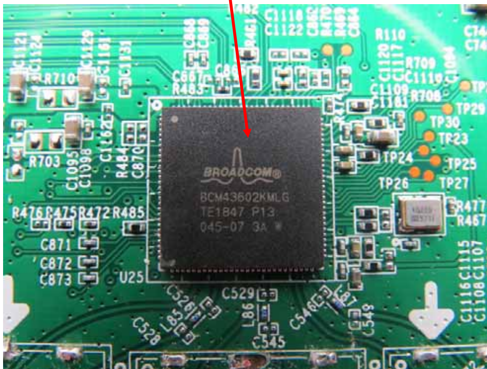
2.4G WIFI RF Chip IC – Top View
