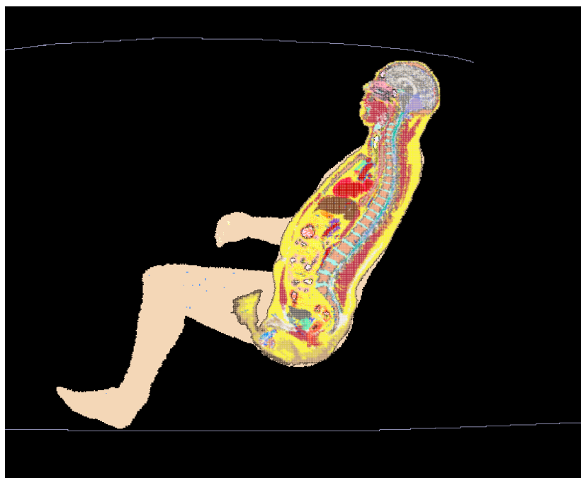
Figure 2: Passenger model exposed to a trunk-mount antenna: XFDTD geometry. The antenna is mounted at 85 cm from the passenger located in the center of the back seat.
