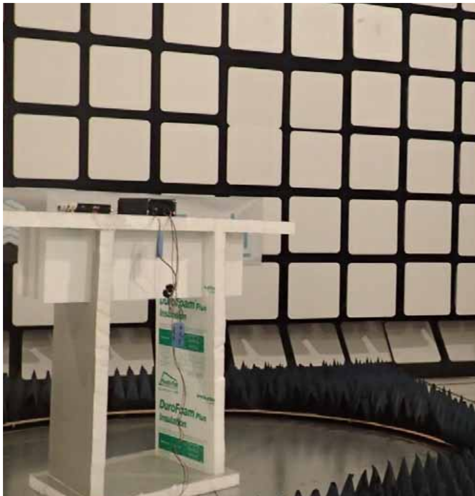
Radiated Emissions at 3 m
