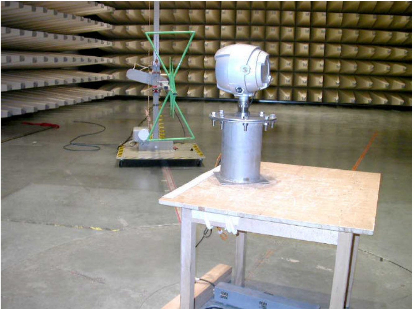
Spurious tests with metal tank
