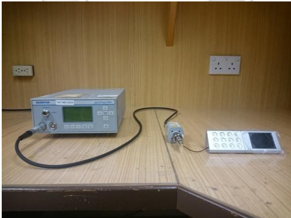
Maximum Peak Power Test Setup
