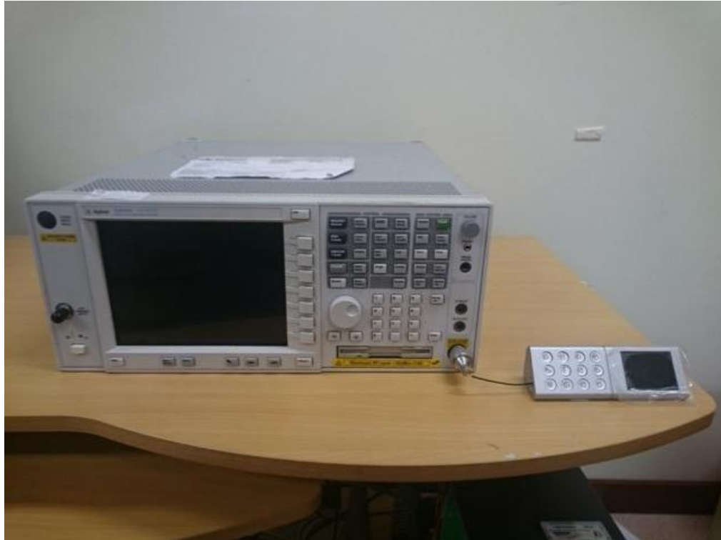
Spectrum Bandwidth (6dB Bandwidth Measurement) Test Setup
