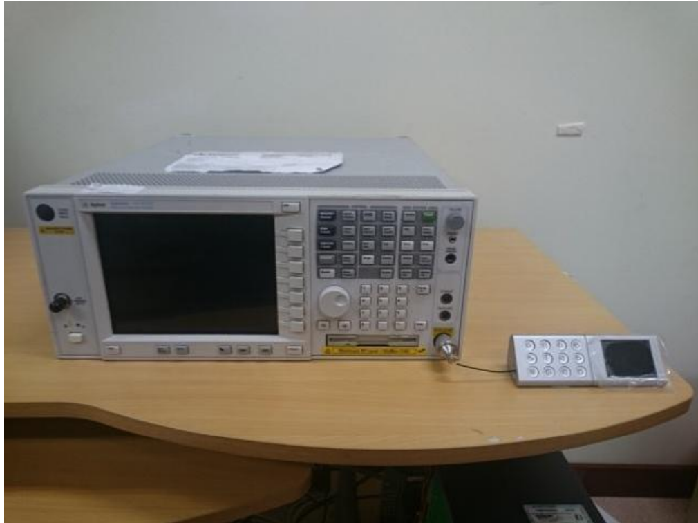
Peak Power Spectral Density Test Setup
