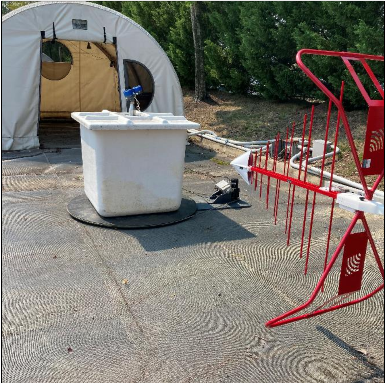
Photograph 7: Radiated Emissions – Fiberglass Container - Front View
