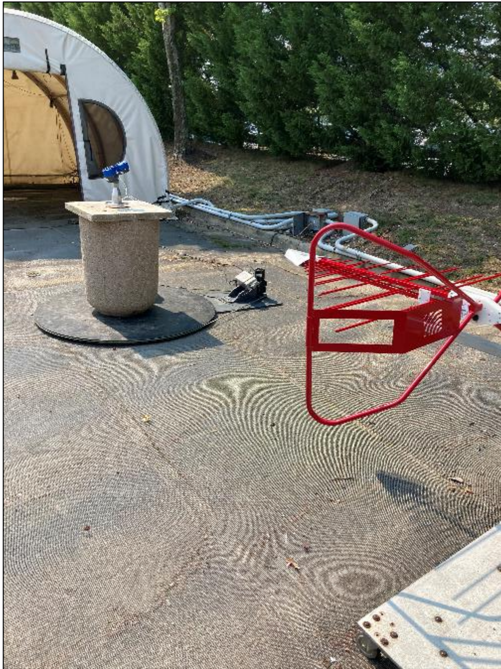
Photograph 3: Radiated Emissions – Concrete Container - Front View
