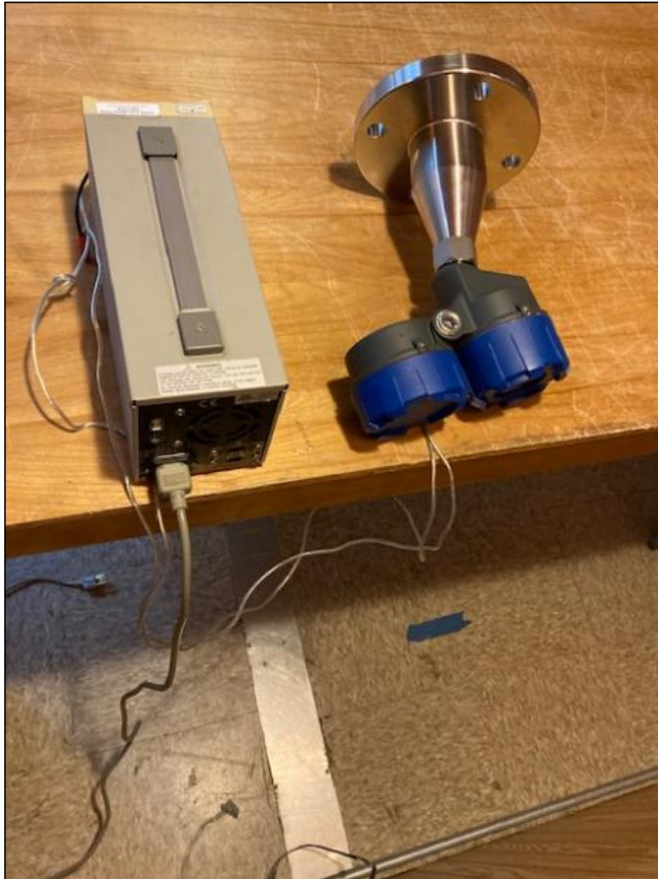
Photograph 4: AC Conducted Emissions - Rear View
