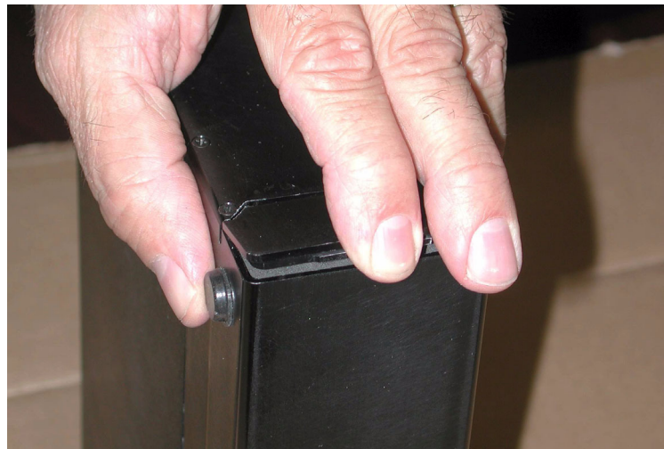
Figure 6-1: Loosening Power/Transceiver Battery Cover
