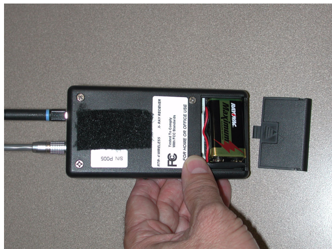
Figure 6-4: X-ray Receiver Battery Location
