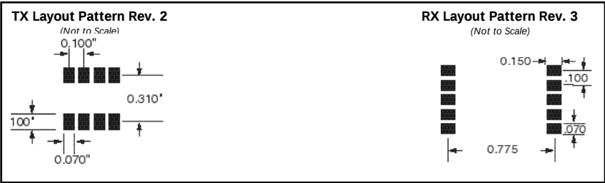
figure 6: Suggested Pad Layout
