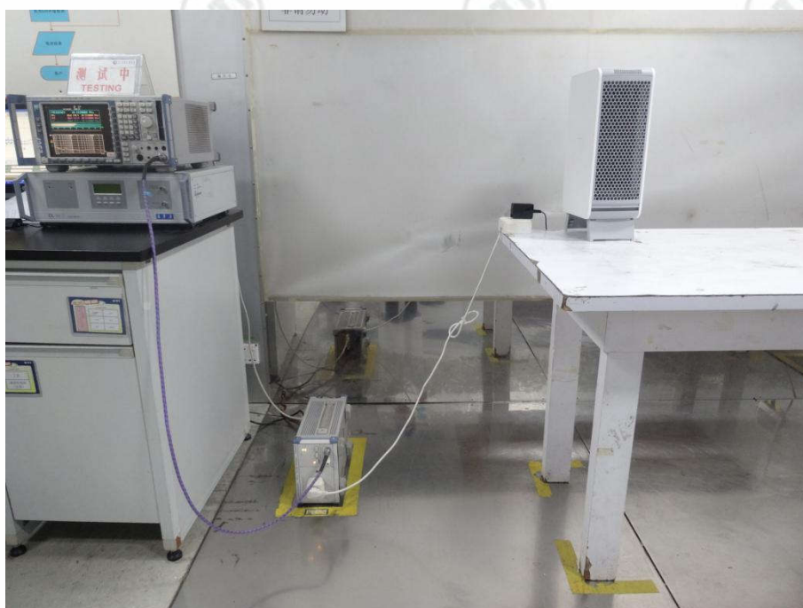
Conducted Emissions Test Setup
