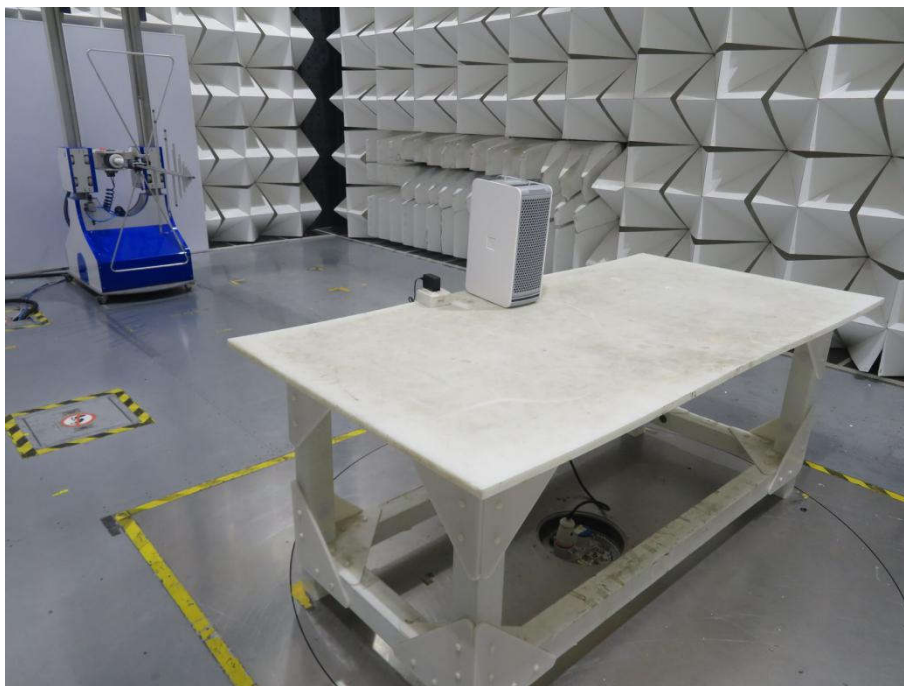
Radiated spurious emission Test Setup-2(30MHz-1GHz)
