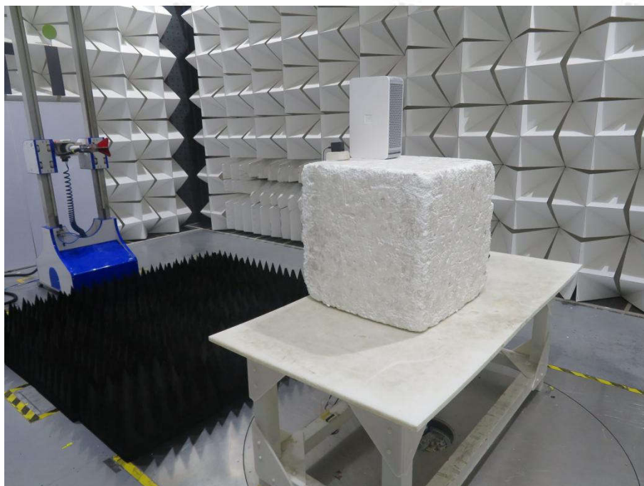
Radiated spurious emission Test Setup-3(Above 1GHz)
