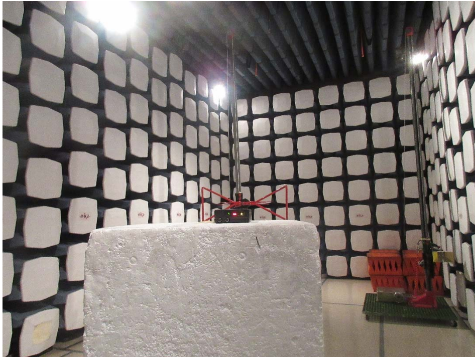
Radiated Emission below 1 GHz (SVR-300M) – Front View
