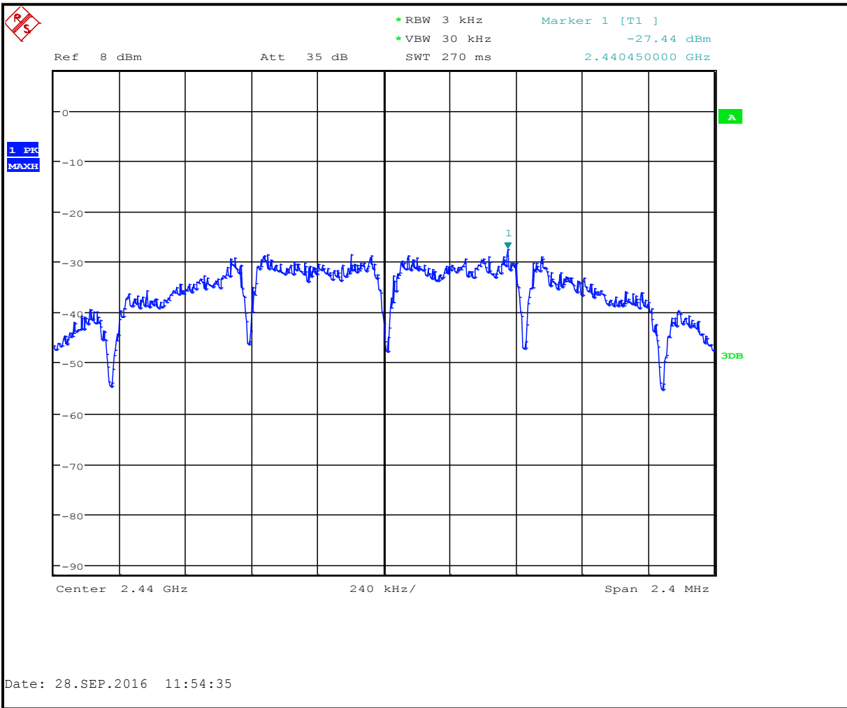
Plot 7-2: Power Spectral Density – 2440 MHz
