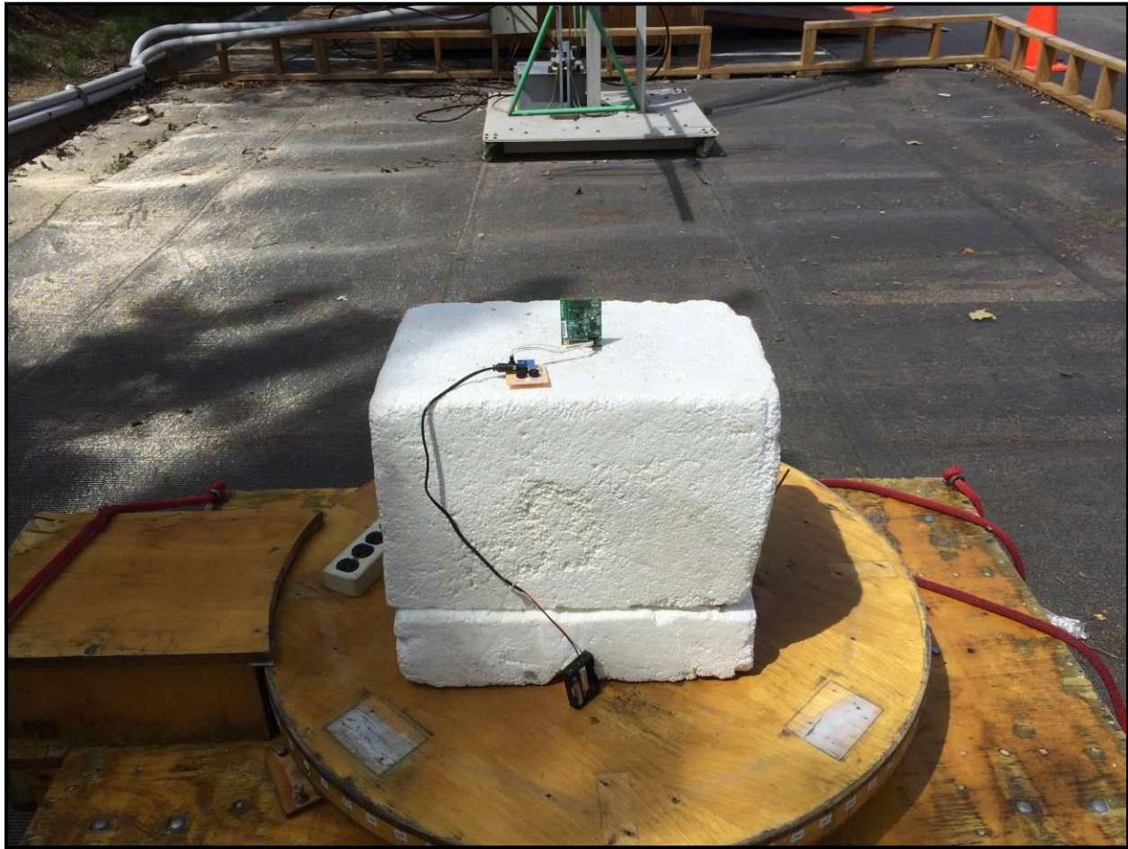
Photograph 2: Radiated Emissions Testing – Front View (< 1 GHz)
