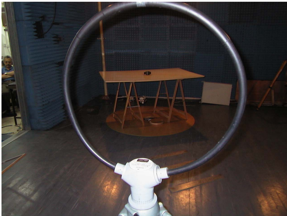
Radiated Emission Test Setup up to 30MHz
