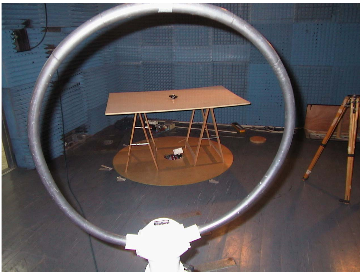
Photo-1 Radiated Emission up to 30MHz
