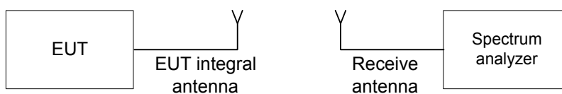
Figure 7.1.1 Setup for transmitter shut down test
