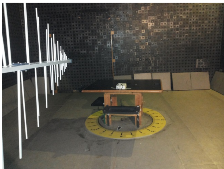
Photograph 8.1.1 Setup for radiated emission measurements
