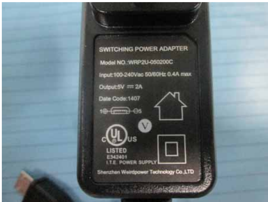
EUT –Adapter#2 Label View
