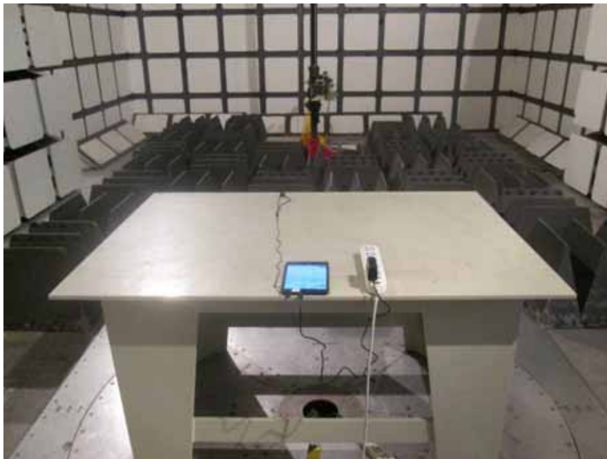
Radiated Emissions - Rear View (Above 1 GHz)
