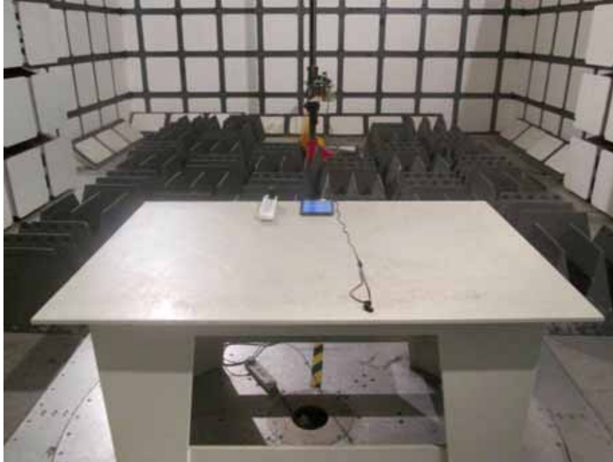
Radiated Emissions - Front View (Above 1 GHz)
