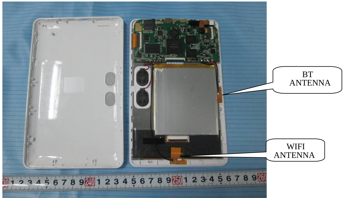
EUT – Cover off View
