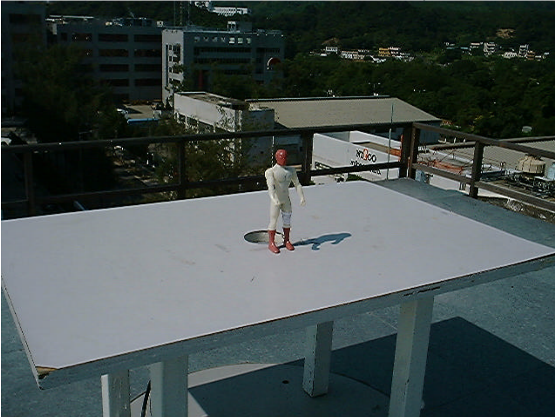
Measurement of Radiated Emission Test Set Up
