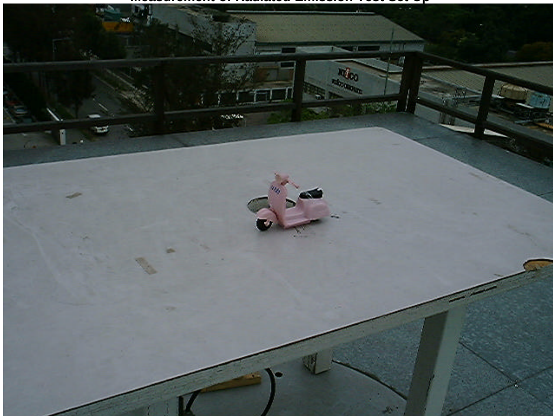
Measurement of Radiated Emission Test Set Up
