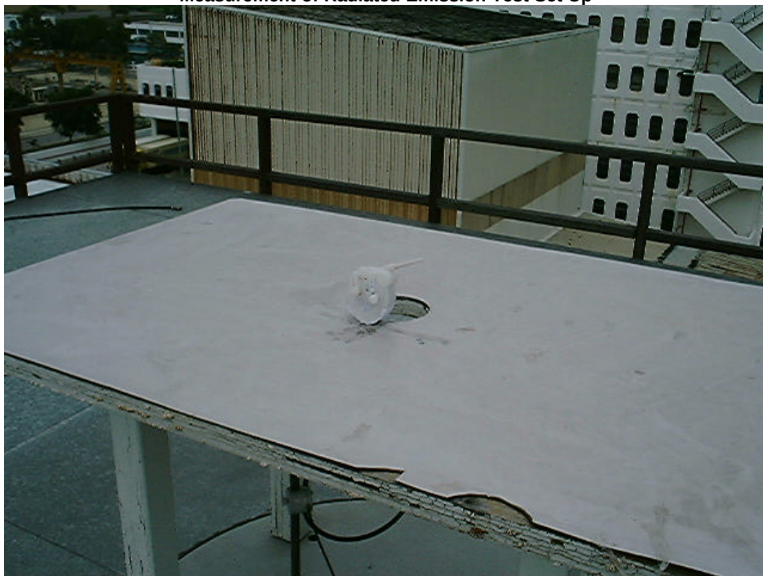
Measurement of Radiated Emission Test Set Up
