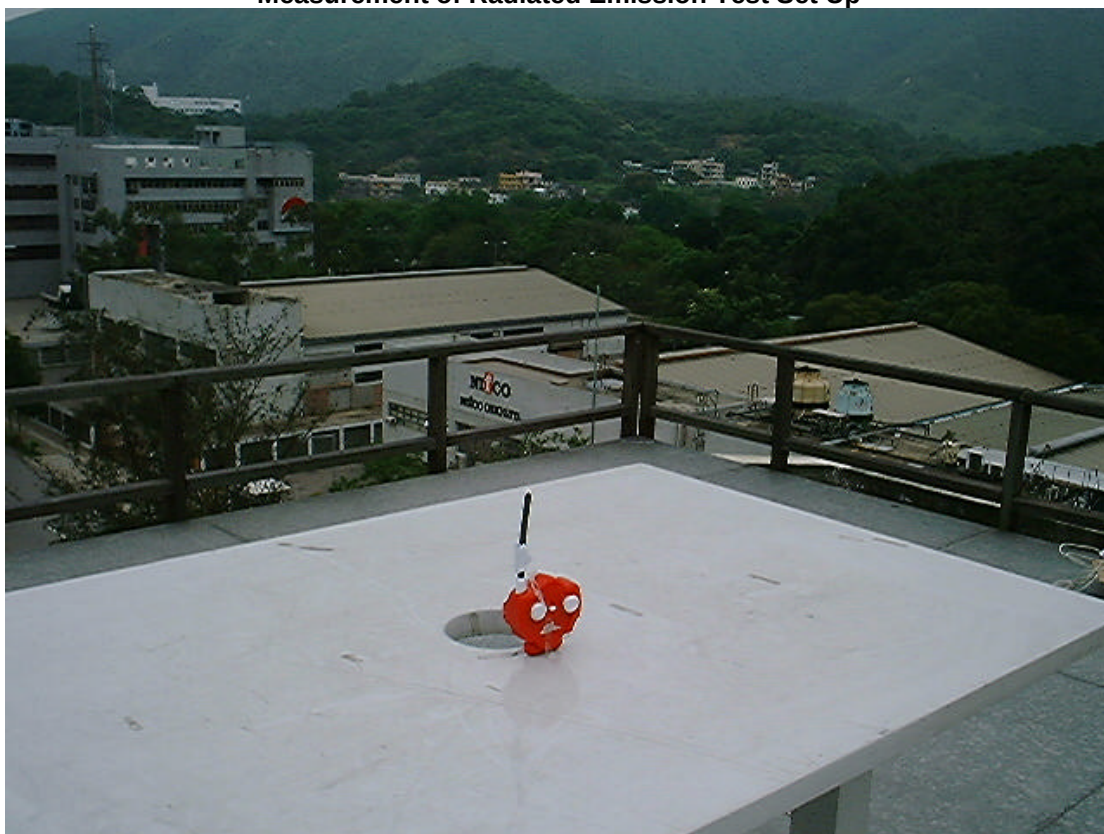
Measurement of Radiated Emission Test Set Up
