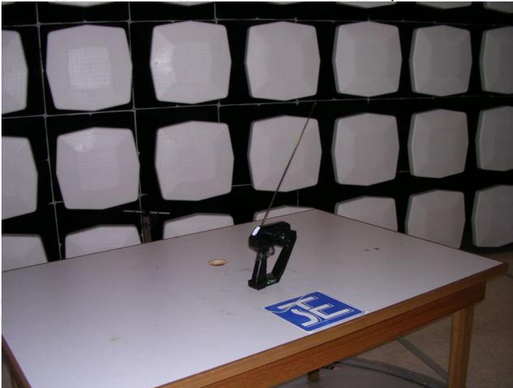
Measurement of Radiated Emission Test Set Up
