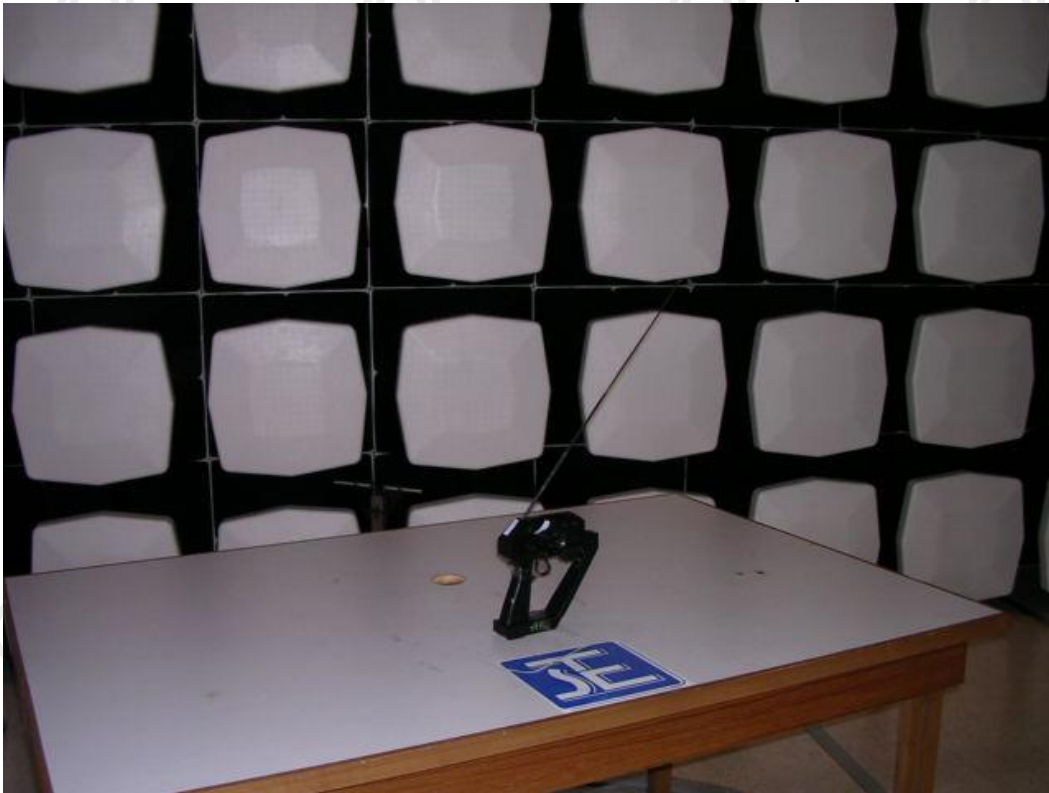
Measurement of Radiated Emission Test Set Up
