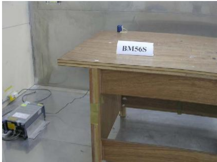
Photo 2: Conducted Emission Test Set-up
