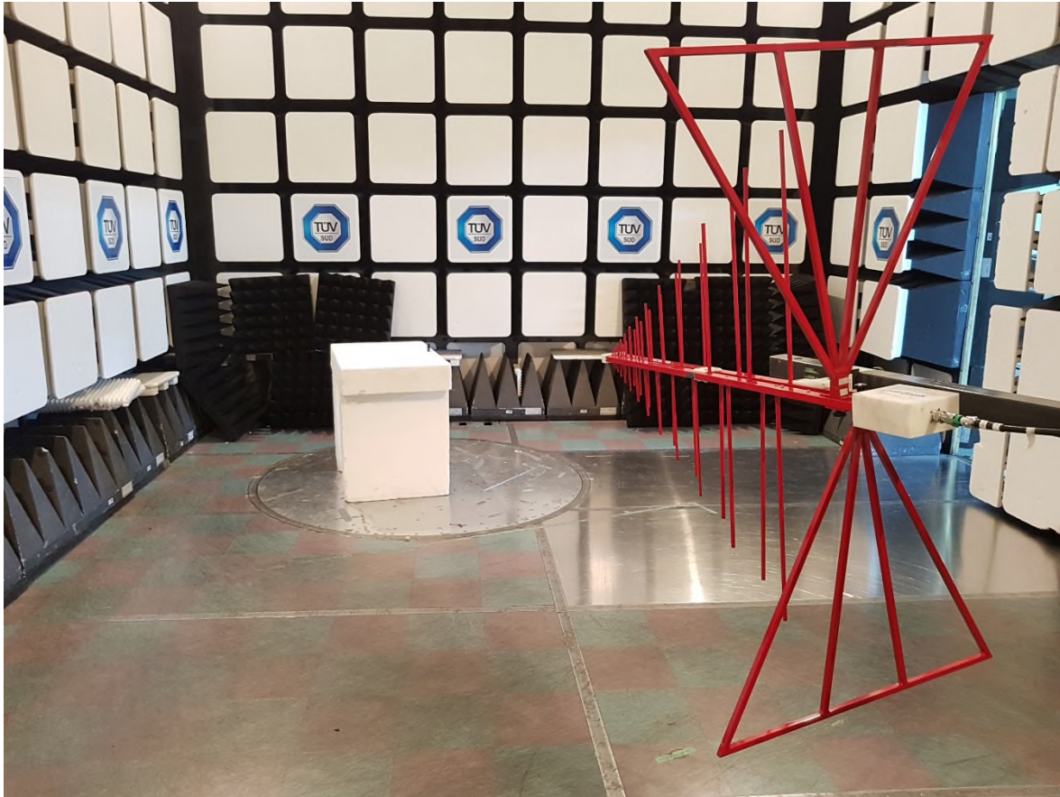
Figure 4 – Radiated Emissions Setup 30MHz – 1GHz
