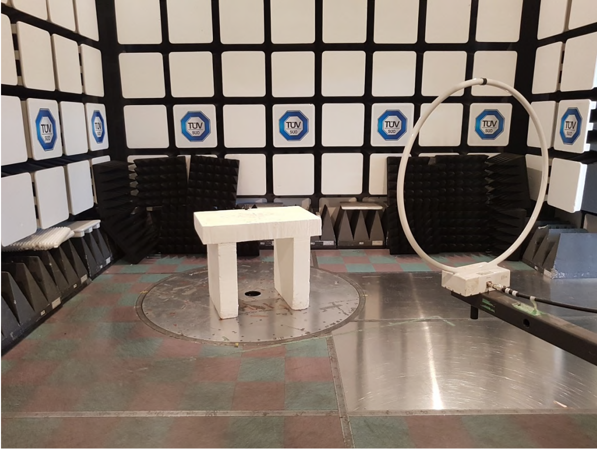
Figure 3 – Radiated Emissions Setup 9kHz – 30MHz
