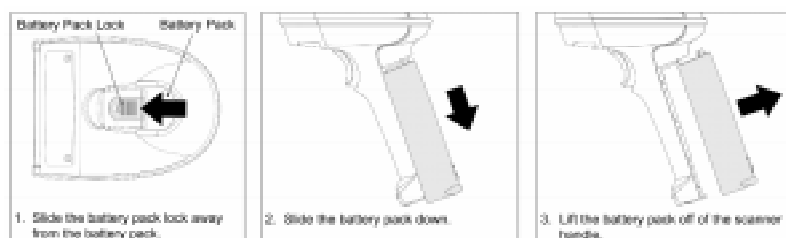
Figure 8. Steps for Removing the Battery for Charging
