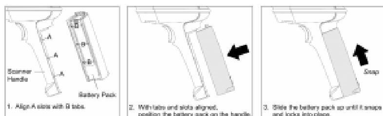
Figure 7. Steps for Installing the Battery
