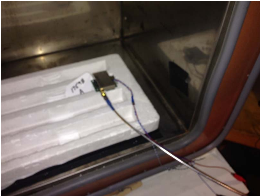
EUT in Temperature Chamber
