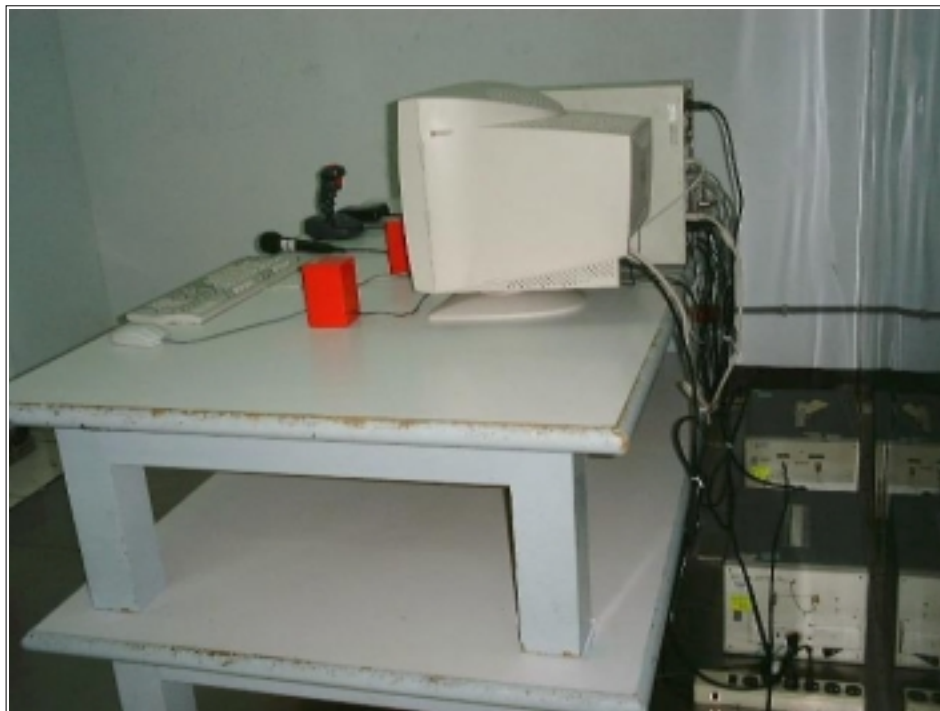
Conducted Emission Setup Photos (Worst Emission Position)
