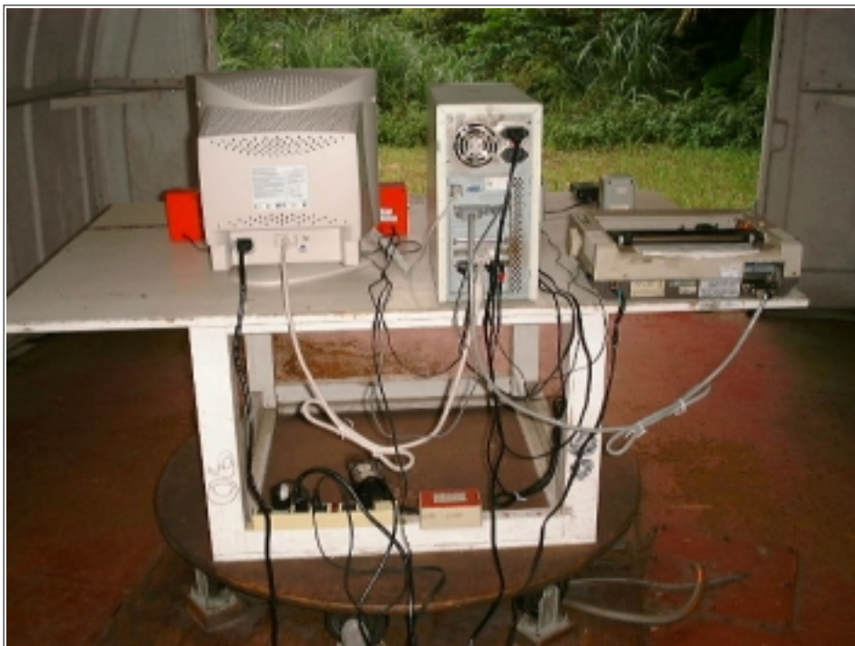
Radiated Emission Setup Photos (Worst Emission Position)
