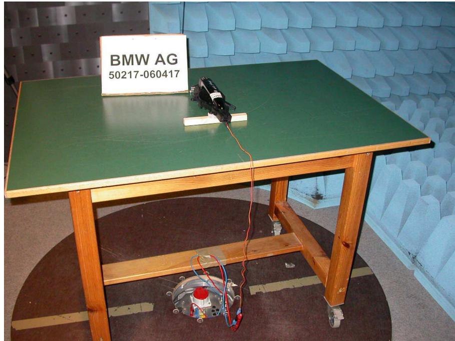
EUT in horizontal position (for prescans only)
