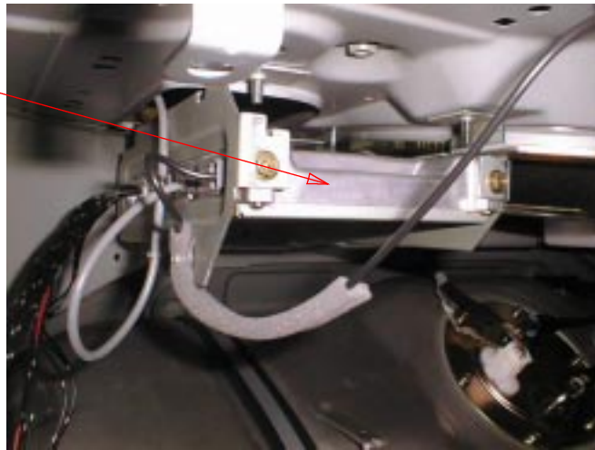
Telematics Communication System (RF Unit / Control Unit )
