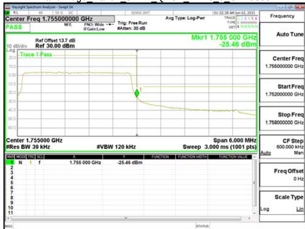
Band Edge Band4 5MHz QPSK RB1 0 CH19975
