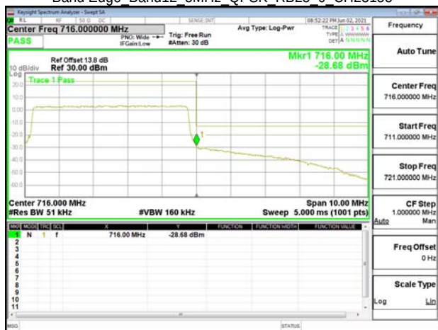
Band Edge Band12 10MHz QPSK RB1 0 CH23060
