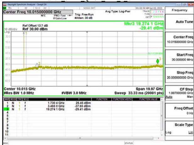
Band4 5MHz QPSK RB1 0 CH20375
