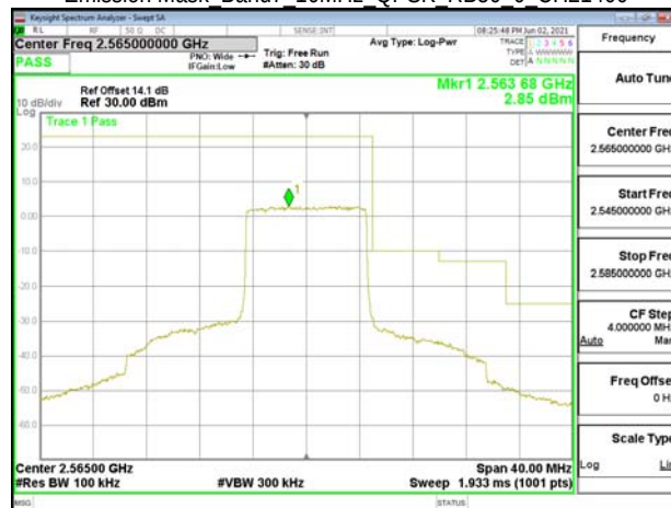
Emission Mask Band7 10MHz QPSK RB50 0 CH21400
