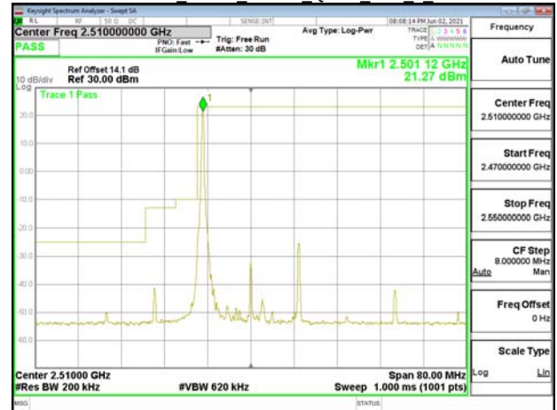
Emission Mask Band7 20MHz QPSK RB1 99 CH21350
