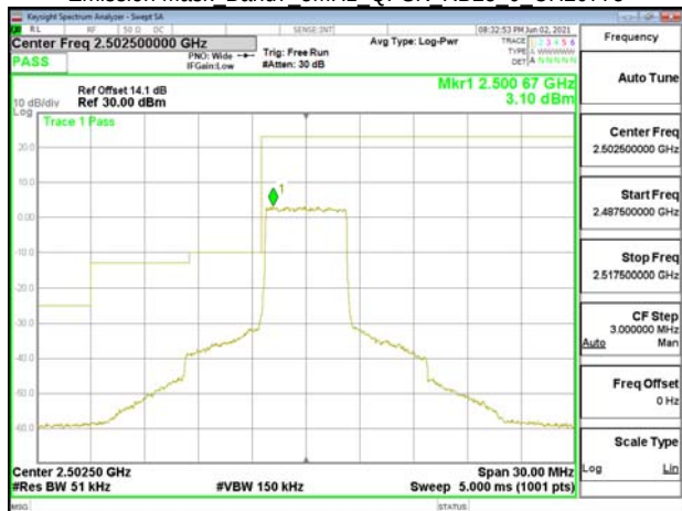
Emission Mask Band7 5MHz QPSK RB25 0 CH21425
