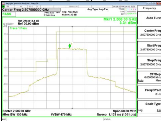
Emission Mask Band7 15MHz QPSK RB75 0 CH20825
