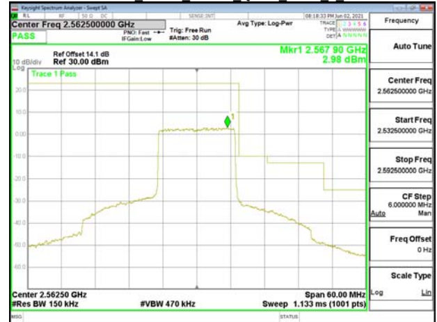
Emission Mask Band7 20MHz QPSK RB1 0 CH20850
