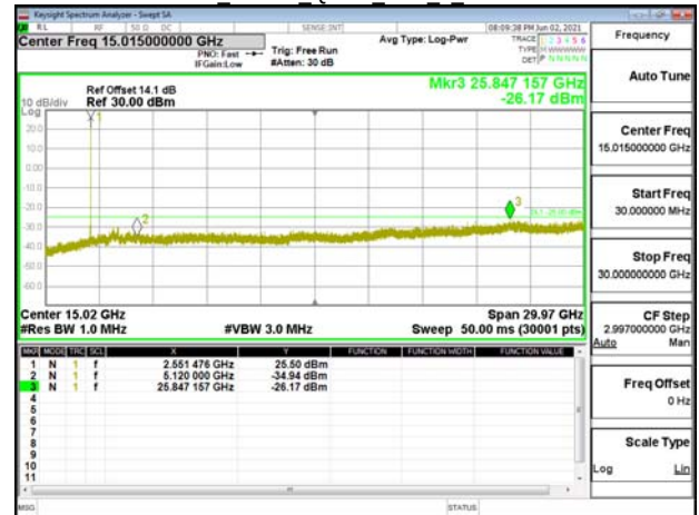
Band7 20MHz QPSK RB1 0 CH21350
