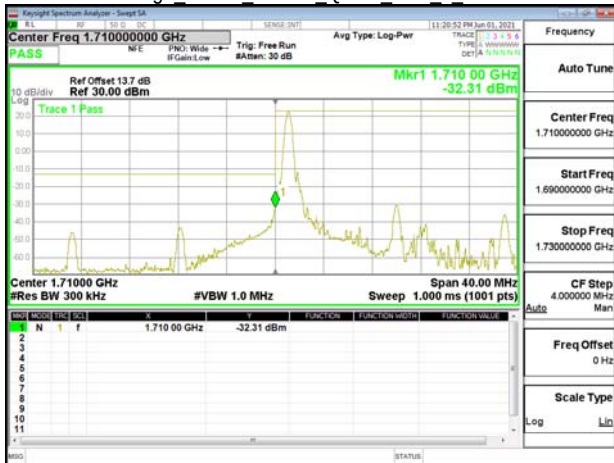
Band Edge Band4 20MHz QPSK RB1 0 CH20050
