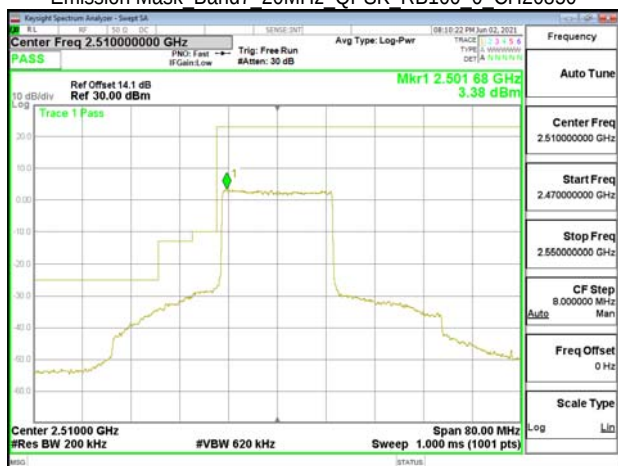
Emission Mask Band7 20MHz QPSK RB100 0 CH21350
