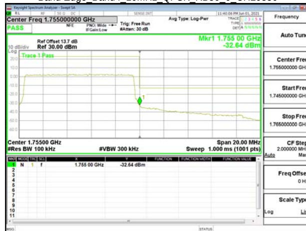
Band Edge Band4 15MHz QPSK RB1 0 CH20025
