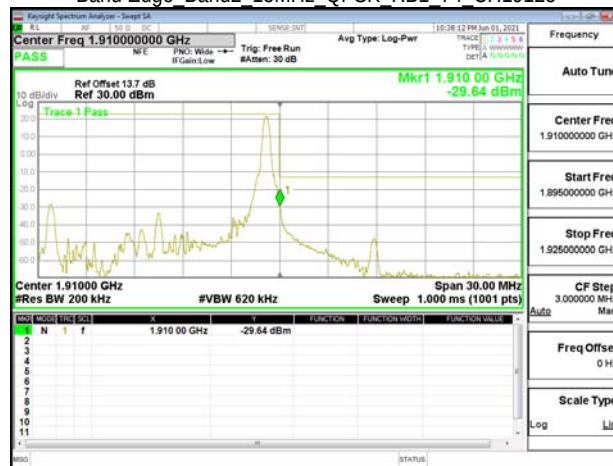
Band Edge Band2 15MHz QPSK RB1 74 CH19125
