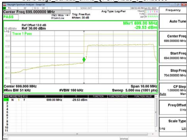
Band Edge Band12 5MHz QPSK RB25 0 CH23155
