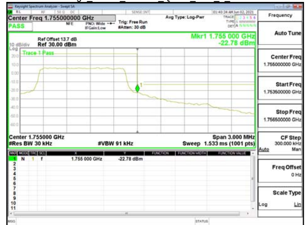
Band Edge Band4 3MHz QPSK RB1 0 CH19965
