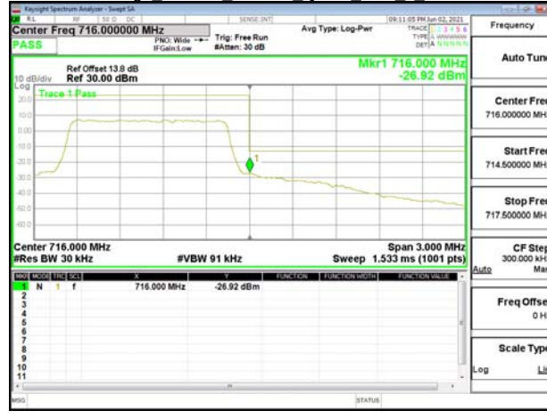
Band Edge Band12 1.4MHz QPSK RB6 0 CH23173
