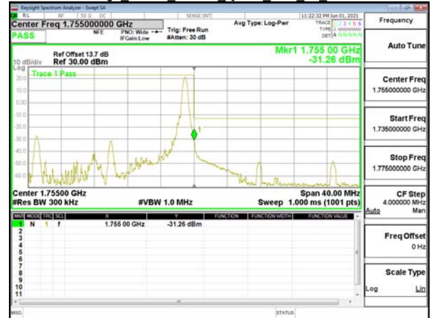
Band Edge Band4 20MHz QPSK RB100 0 CH20050
