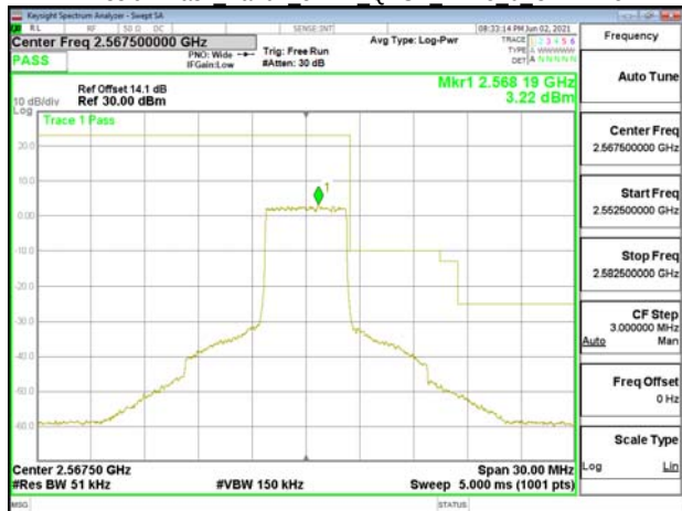
Emission Mask Band7 10MHz QPSK RB1 0 CH20800
