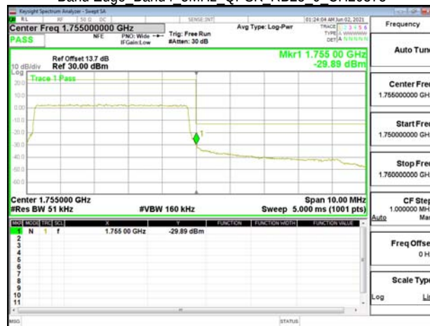
Band Edge Band4 5MHz QPSK RB25 0 CH20375
