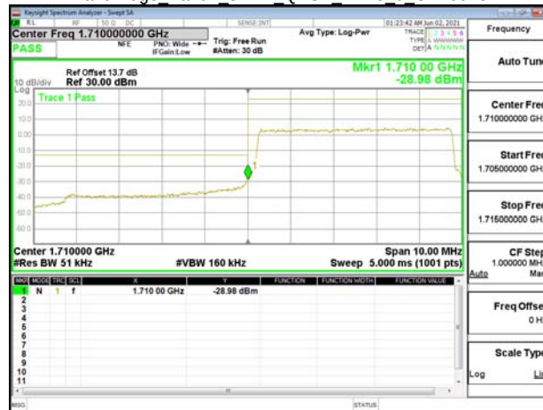
Band Edge Band4 5MHz QPSK RB25 0 CH20375
