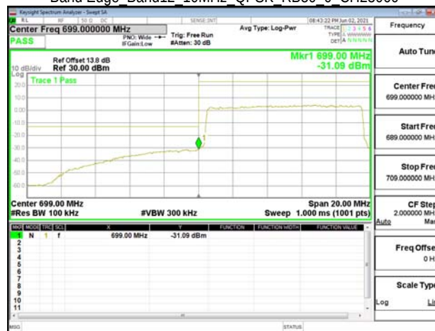
Band Edge Band12 10MHz QPSK RB50 0 CH23130
