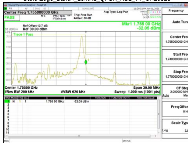
Band Edge Band4 15MHz QPSK RB1 74 CH20325
