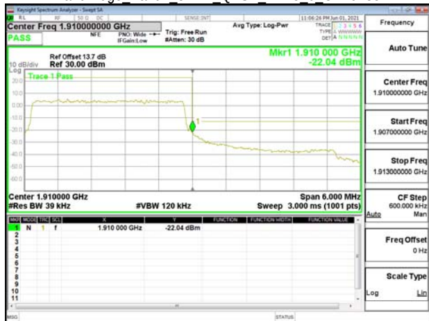
Band Edge Band2 5MHz QPSK RB1 0 CH18625
