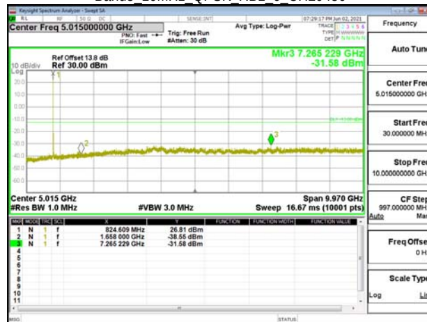
Band5 10MHz QPSK RB1 0 CH20525
