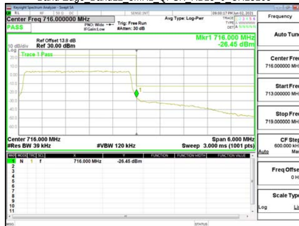
Band Edge Band12 5MHz QPSK RB1 0 CH23035
