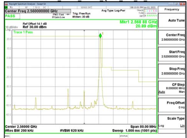
Emission Mask Band7 20MHz QPSK RB1 99 CH21350
