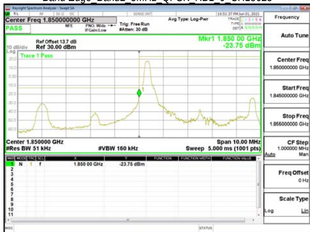
Band Edge Band2 5MHz QPSK RB1 0 CH18625
