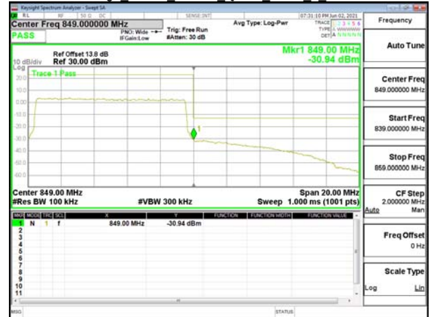
Emission Mask Band7 5MHz QPSK RB1 0 CH20775
