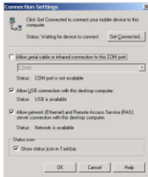
Figure 6.43 Disconnect SPP connection in Microsoft's ActiveSync
