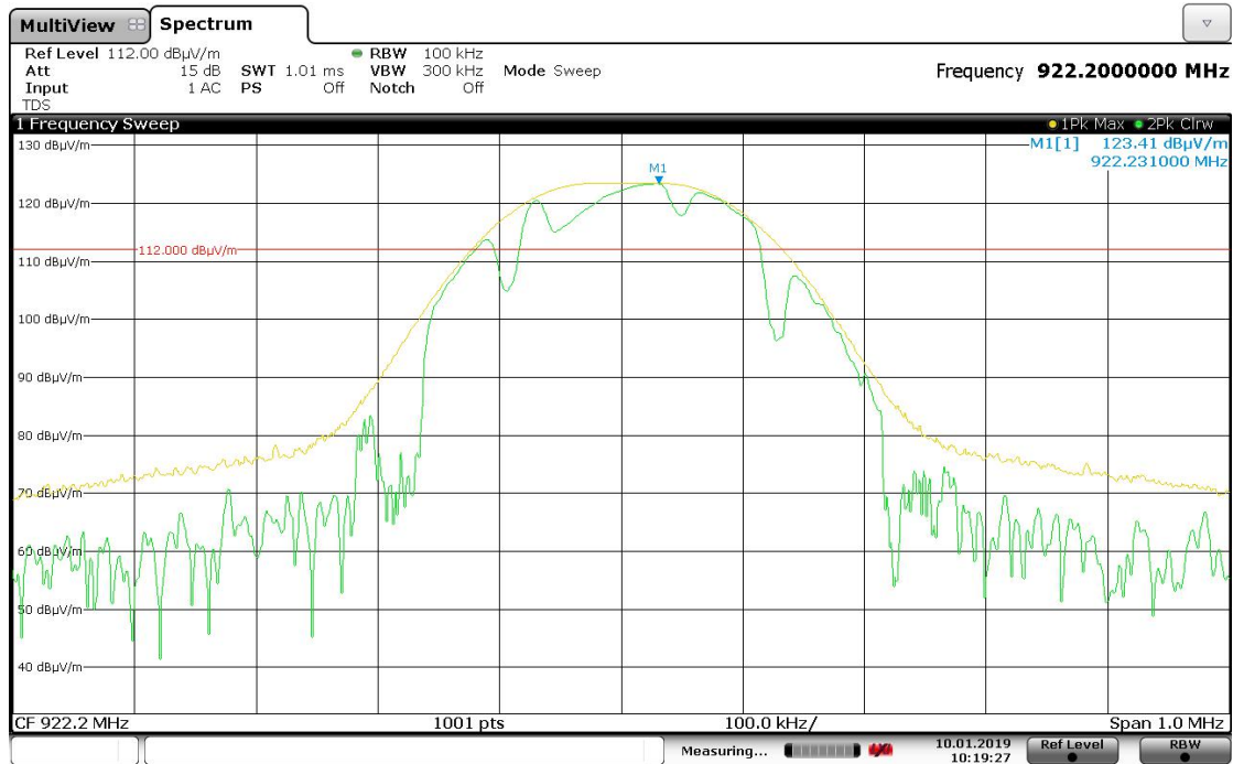
Graph 6-10: 100 kHz bandwidth. Peak measurement, EUT x-axis, Measurement antenna – Vertical polarisation, Middle channel – 922.2 MHz
