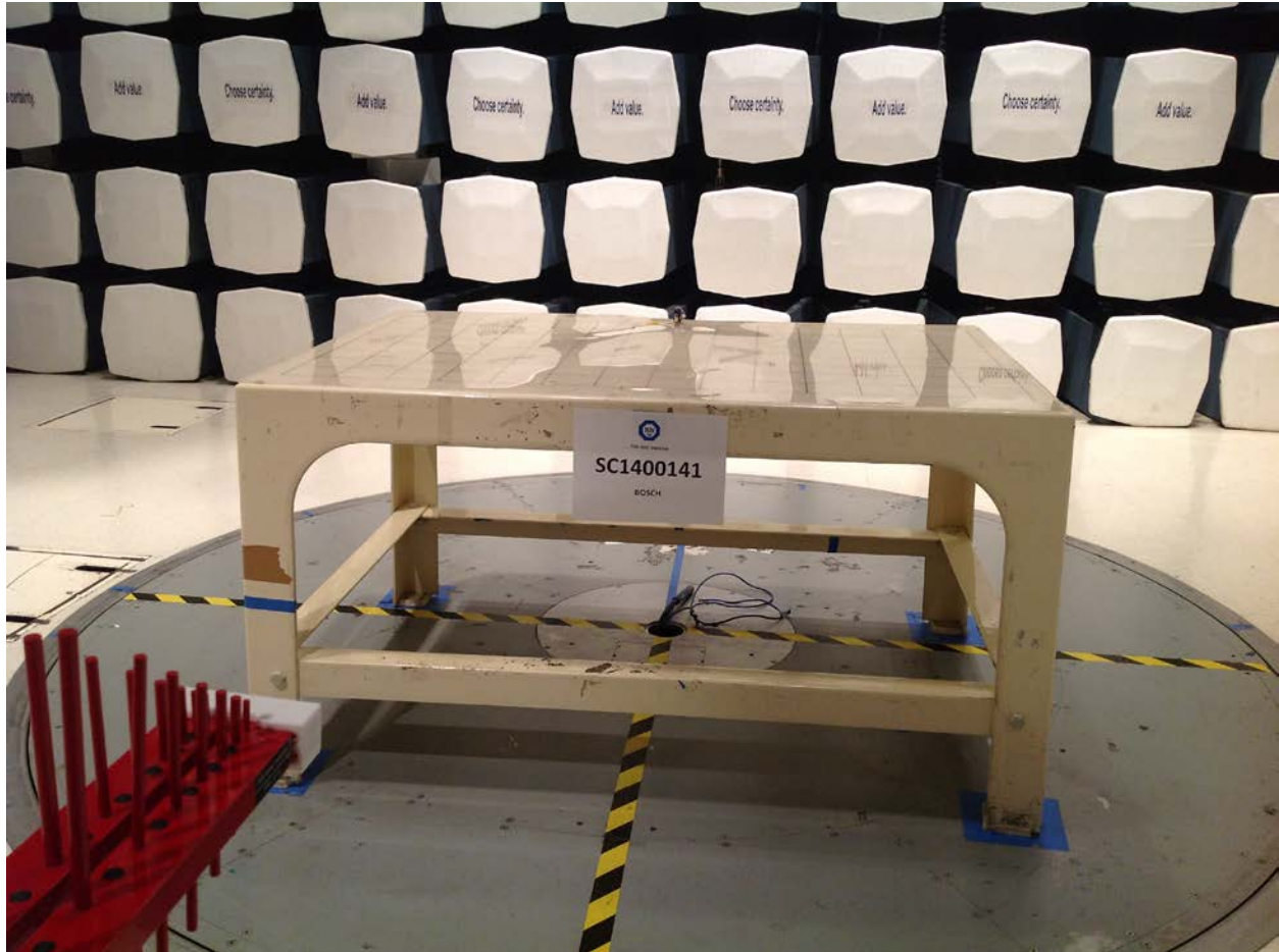
Radiated Emissions Test Setup (<1GHz)
