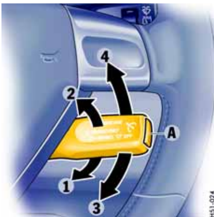
A - Automatic speed control readiness off/on 1 - Hold and store/accelerate 2 - Decelerate/resume 3 - Interrupt
