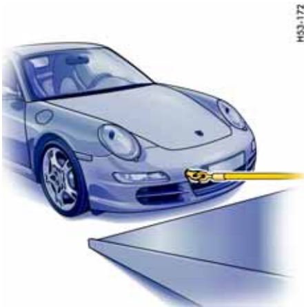
Pulling vehicle onto flat bed
