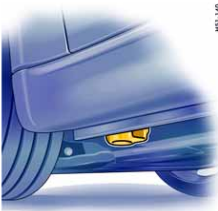
A - Front jacking point
