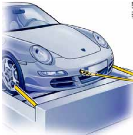
Tieing down vehicle on flat bed
