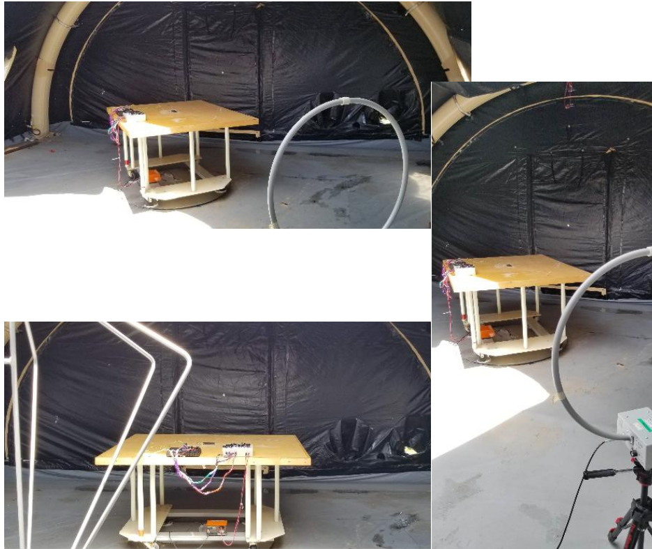
Figure 4: Radiated Emissions Test Setup Photograph(s).
