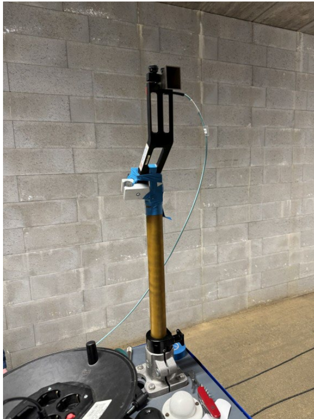
Photo 5: Standard gain horn 18 GHz – 26.5 GHz on trolley
