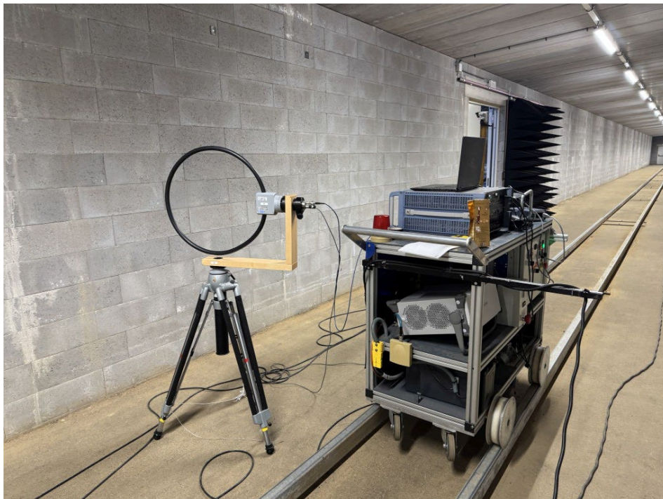
Photo 7: HFH2-Z2 magnetic field antenna 9.0 kHz – 30 MHz
