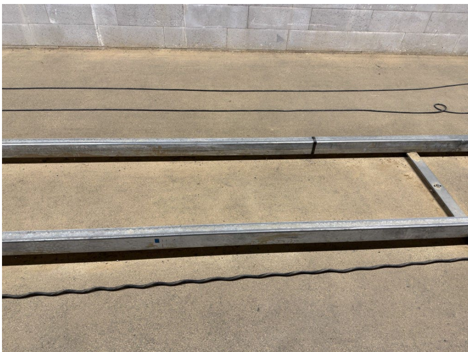
Photo 4: Tracks on the floor for the trolley, with marks for worst-case positions
