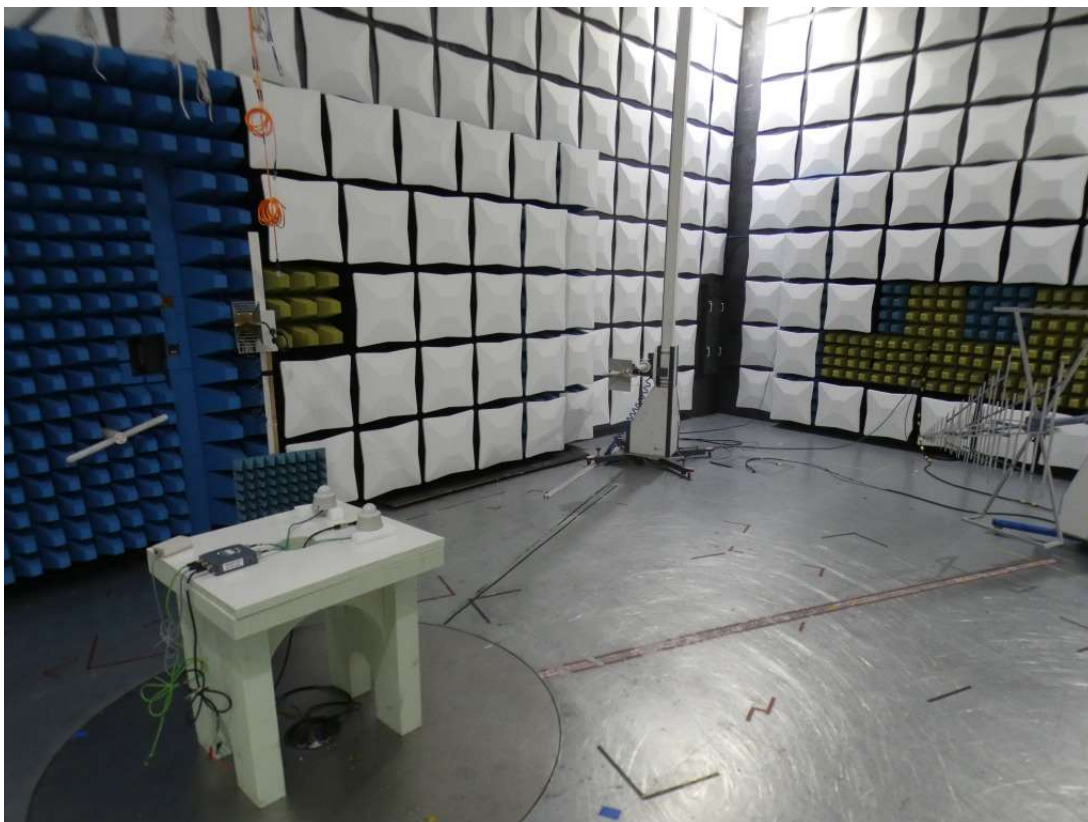
Photo 8: Test setup for radiated emissions measurements in semi-anechoic chamber (30 MHz to 1 GHz), right side view, [Setup S04_AJ01]
