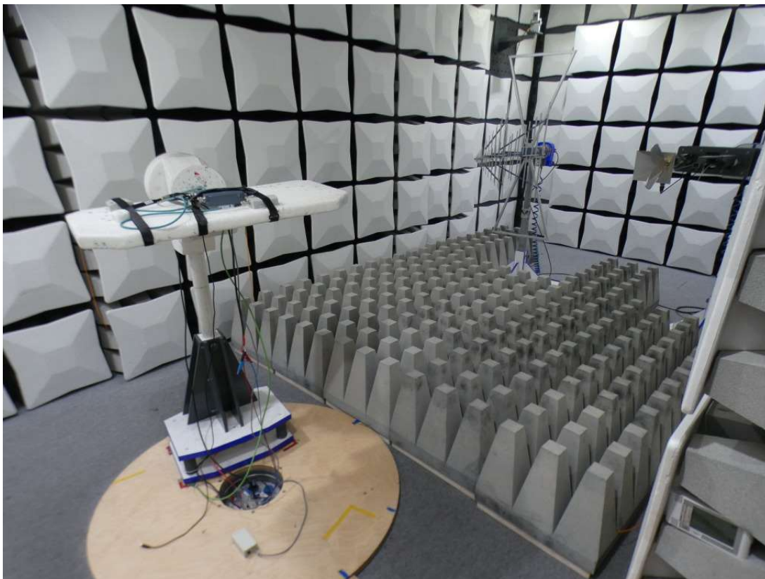
Photo 9: Test setup for radiated emissions measurements in fully -anechoic chamber (1 GHz to 26 GHz), right side view, [Setup S03_AJ01]
