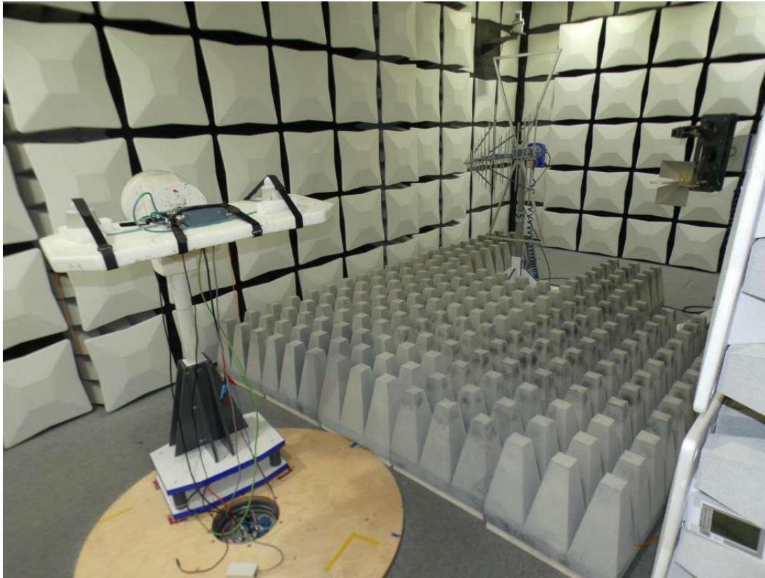
Photo 8: Test setup for radiated emissions measurements in fully -anechoic chamber (1 GHz to 26 GHz), right side view, [Setup S04_AJ01 ]
