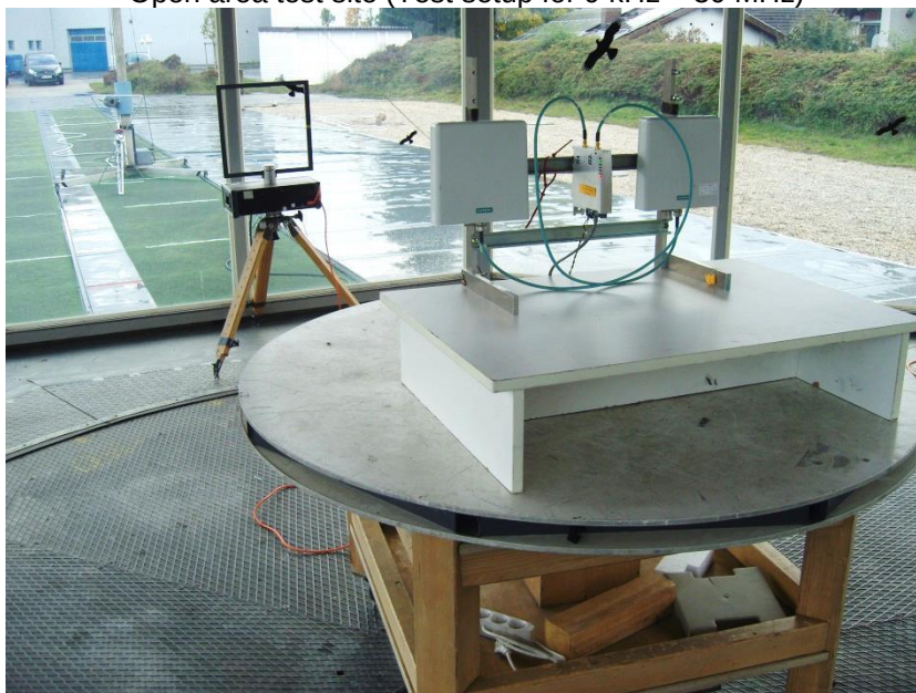
Open area test site (Test setup for 9 kHz – 30 MHz)
