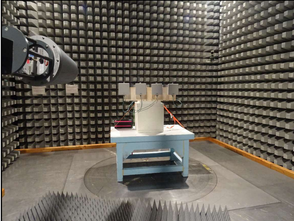
Photo 54: EUT- MIMO PORT 1+2+3+4 (No Port Terminated with 50 \Omega )
