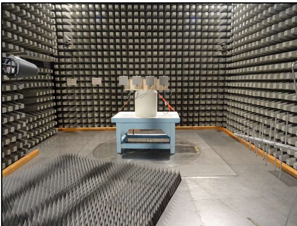
Photo 57: EUT- MIMO PORT 1+2+3+4 (No Port Terminated with 50 Ω)
