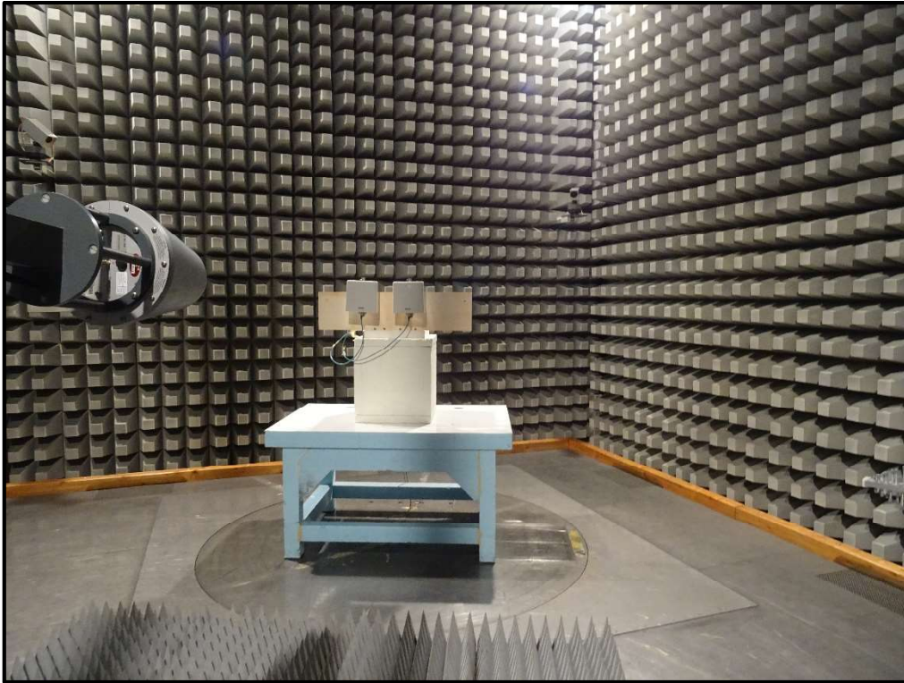
Photo 49: EUT- MIMO PORT 1+2 (Ports 3 & 4 Terminated with 50 \Omega )
