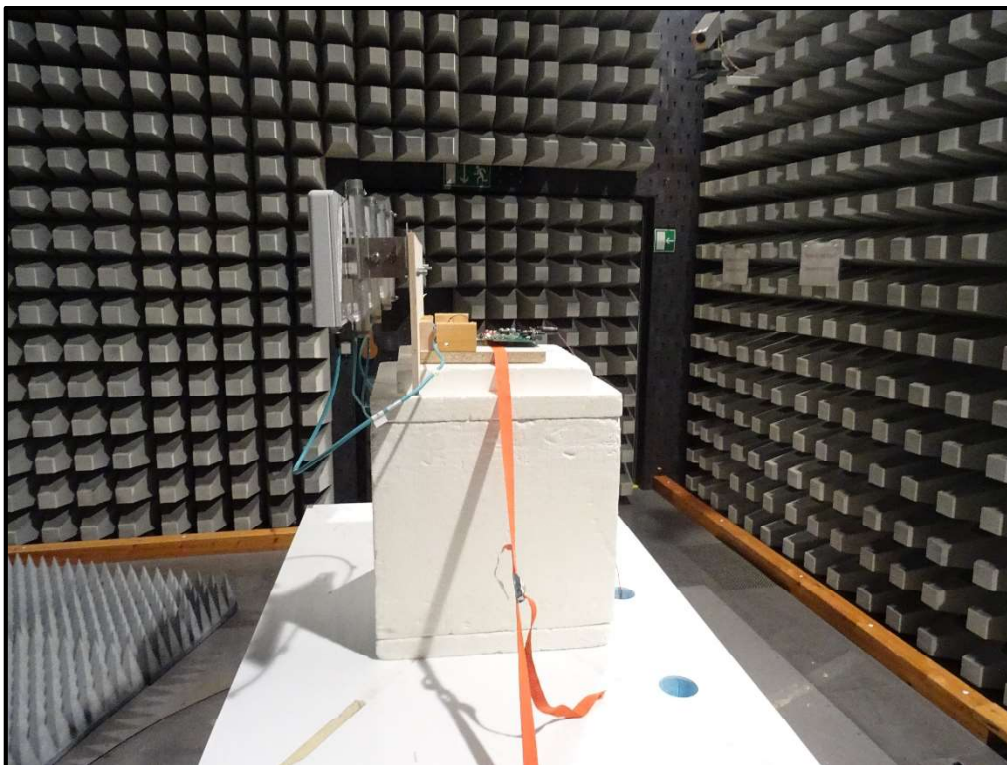
Photo 56: EUT- MIMO PORT 1+2+3+4 (No Port Terminated with 50 Ω)
