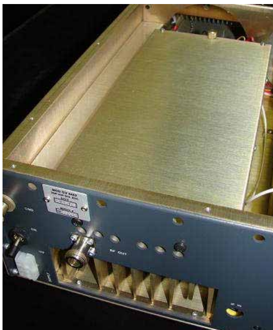
Fig.3.9: Module 20W UHF ATSC power amplifier – module 4464
