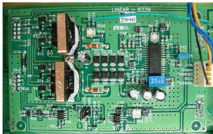
Fig.5.9: CIM3429 – Full Bridge Control PCB.
