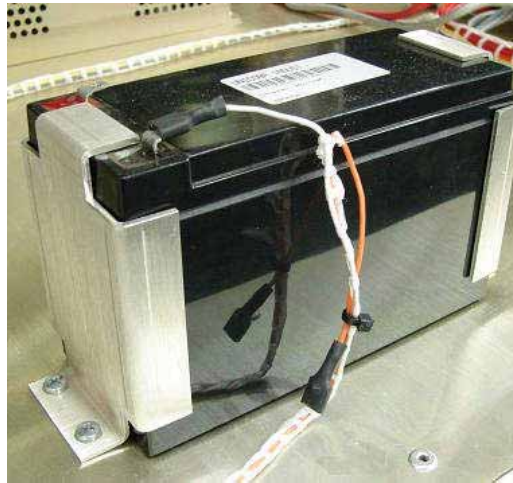
Fig.7.10: 12V/7AH Battery – shown with + cable disconnected
