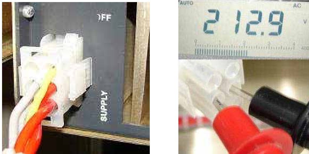
Fig. 7.6: On the right the drawer AC power connector, on the right AC mains reading on the center pins of the same connector.
