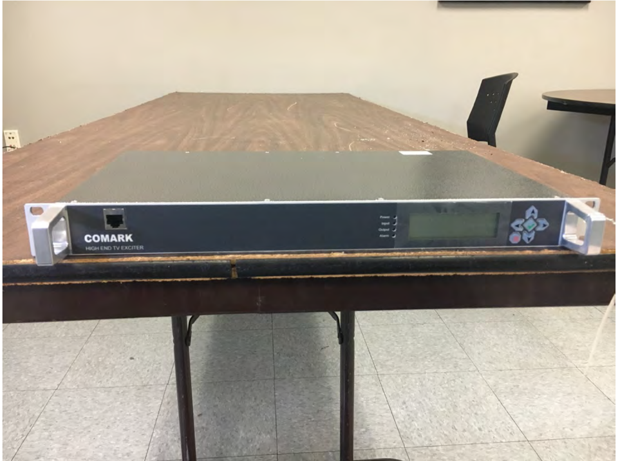
Figure 3. Exact V2 Exciter Front View
