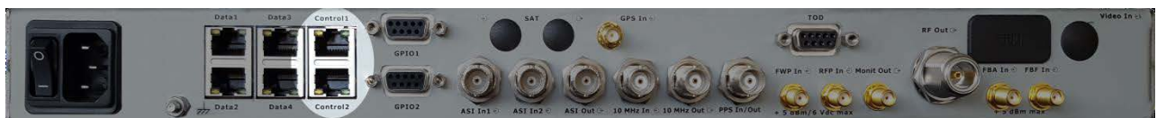
Figure 27: Electrical Gigabit Control Interfaces
