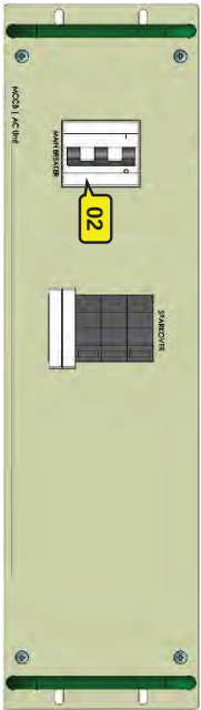
MCCB AC Mains T220 / T380 (Front View)
