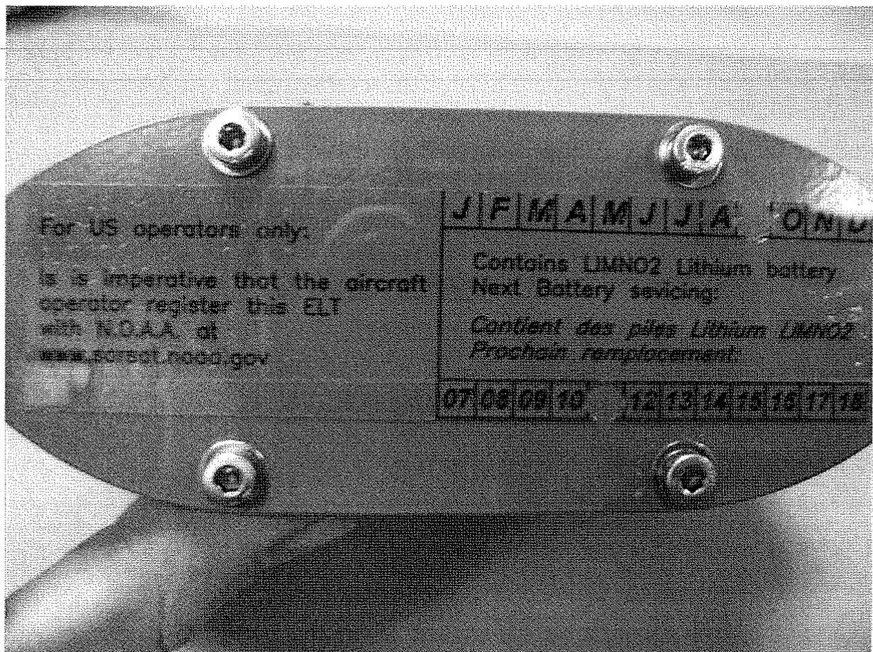
Batteries servicing label and note for US registration label on ELT model ADT 406 S
