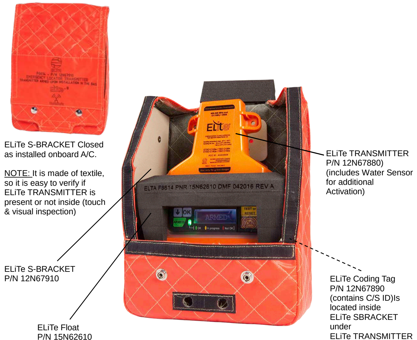
Figure 4 Survival – ELiTe S-BRACKET Sub Components
