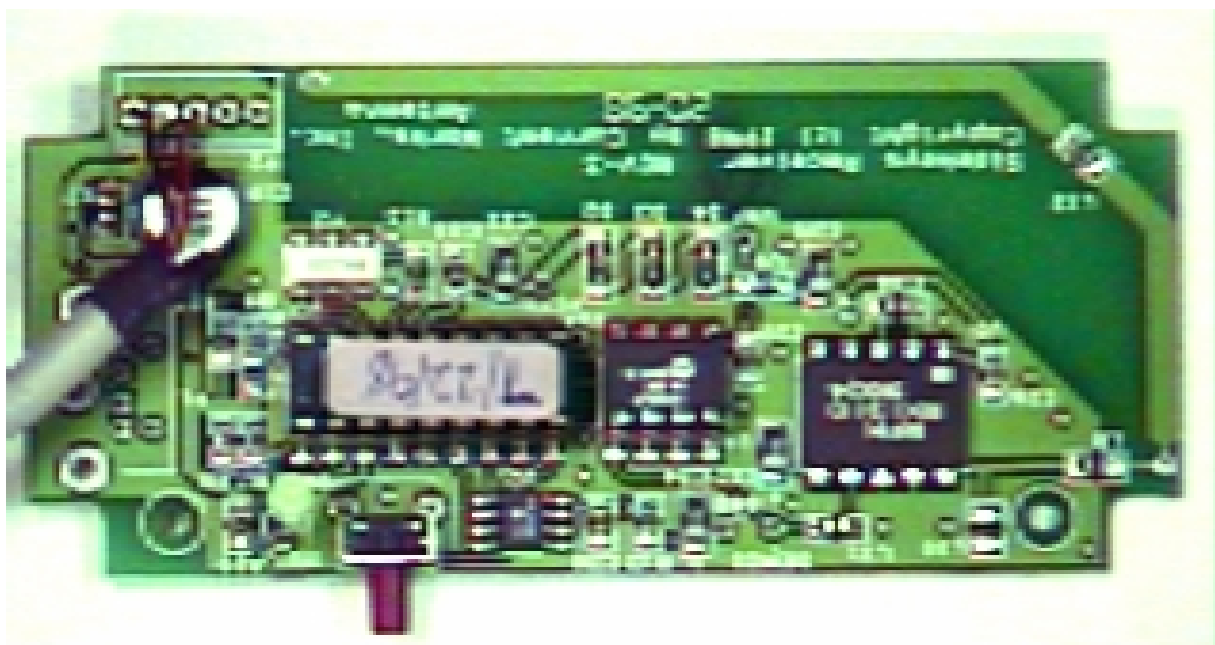
Component side of Receiver PCB
